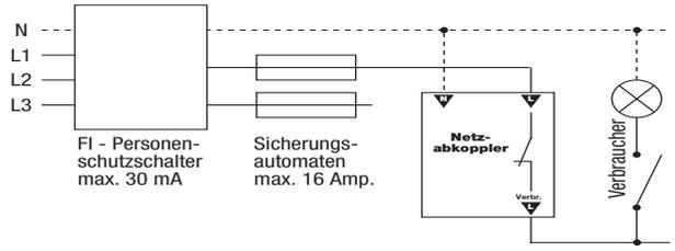
Switch off the Main Switch for the electricity supply before installation. Connect input "N" with the neutral conductor bar and input "L" with the output of the desired circuit breaker. Switch on the main switch.
