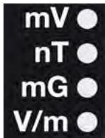
In general, the display will show the three dimensional (“resulting”) magnetic field. There is no need for a conversion: Simply read the measurement value on the display and the unit on the LEDs. The signal of an AC/DC input possibly connected to the device will be shown in millivolt. Use the key “^” to switch from one display mode to the other.
